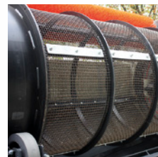
Screen drum Adjustable speed 0-20 RPM
