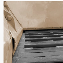
Feeder Plate apron feeder for wet sticky material, heavy rock, high fines.
