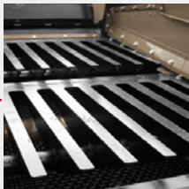
Large rock Top deck grizzly bars for very rocky application.
